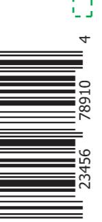
It is recommended that all barcodes be placed vertically, never horizontally as the bars may distort with the transverse shrink.
